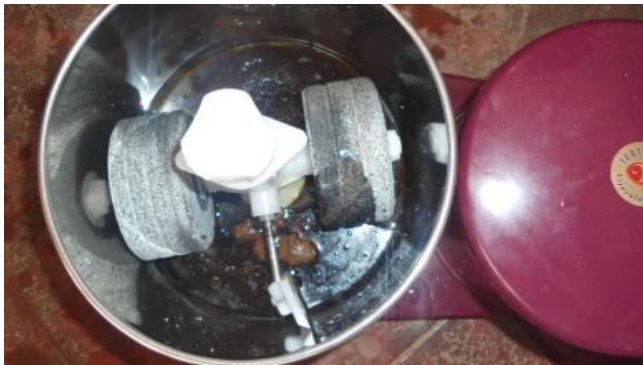
3 rd sample: Mixing the ingredients all together using edge runner mill
