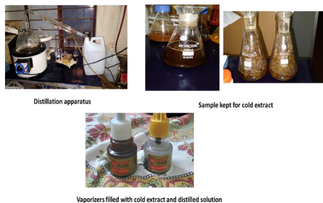
Figure 2: Few representative images showing the - a) Distillation apparatus, b) sample kept for cold extract and c) vaporizers filled with cold extract and distilled solutions.
