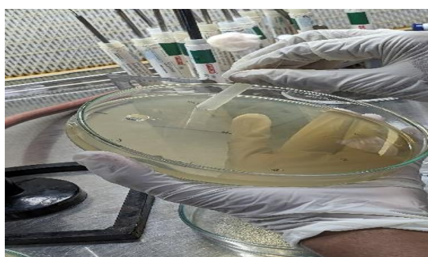
Fig 2: B) Opening wells with upside-down plastic tips
