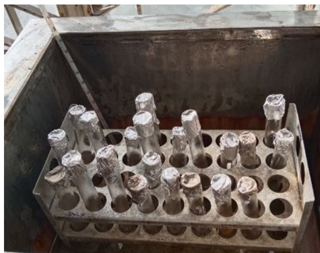
Figure 2.c: Incubation of reaction mixtures in water bath
