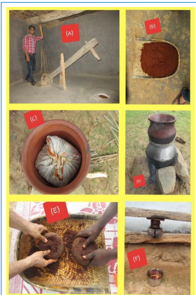
Figure 3: Procedure of Oil extraction by traditional method (a) Crushing of seed, b) crushed seeds, c) Crushed seed tied in Cotton cloth, d) Steaming, e) Steamed seeds Filling in Pottali , f) Pressing by Tirhi
